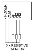
Standard connection of three resistive sensors to analog inputs.
