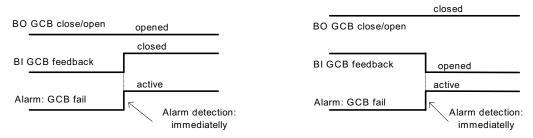
When BO GCB close/open (MCB close/open) opens there is 5 sec delay for GCB fail (MCB fail) detection.
