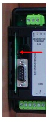
RS 232 communication module with the boot jumper.
