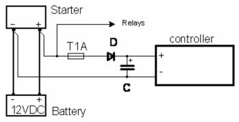
The capacitor size depends on required time. It shall be approximately thousands of microFarads. The capacitor size should be
