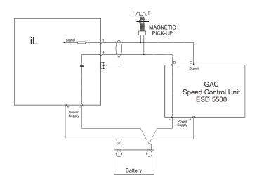
Be aware of interference signal from Speed governor when one speed pick-up is used. If engine will not start:
