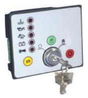
During engine cranking and for a short time afterwards the **protection hold-off timer** (10 seconds) is active and the relevant alarm inputs are inhibited. This enables the engine to start and achieve normal running conditions. Once the timer has expired the inputs are enabled providing normal protection from the module.
