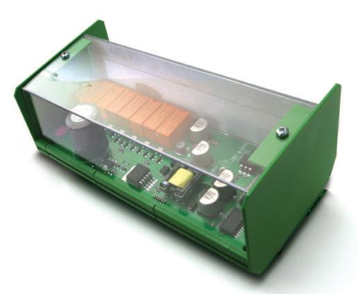
The DSE157 is an output relay expansion module for use with DSEControl® and DSEPower® Series Modules (excluding DSE51xx).
