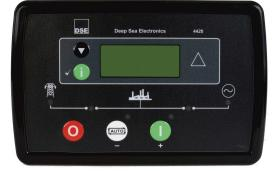
The DSE4410 is an Auto Start Control Module and the DSE4420 is an Auto Mains (Utility) Failure Control Module for single gen-set applications. Both modules have been designed to work with electronic and non electronic engines providing advanced engine monitoring and protection features.
