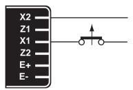
The exciter is switched off by disconnecting the AVR power supply (1 wire - X1 or X2). Contact rating 16 A - 250V A.C.
